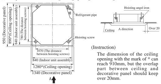
(2) If necessary, cut the opening installation needed in the ceiling. (For the condition of having ceiling)
